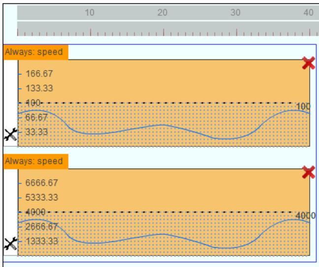
Fig. 7: Example 6: The graphical formalism for the MTL specification  $\phi_6 = (\Box_{[0,40]}(speed < 100)) \wedge (\Box_{[0,40]}(rpm < 4000))$ .
